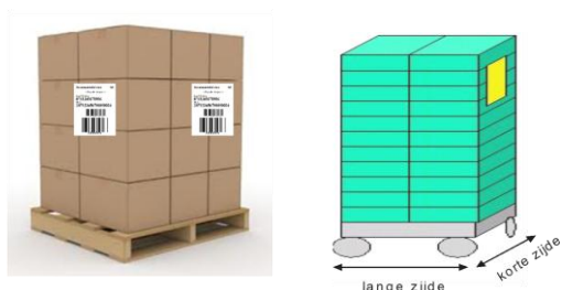
Figure 6.1: Position of GS1-labels on pallets and trolleys
